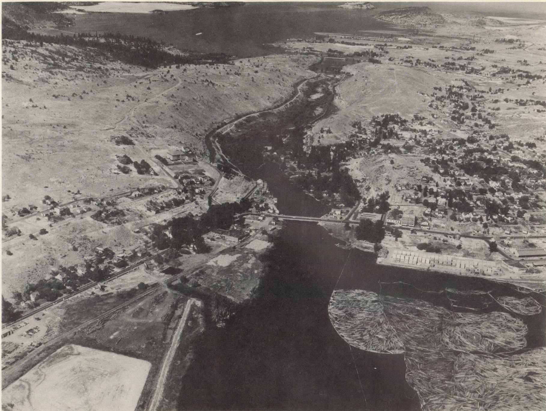
Link River, about one mile long, showing Lake Ewauna in foreground, upper Klamath Lake in background and a part of the city of Klamath Falls. The picture shows the dam at the outlet of Upper Klamath Lake and the power conduits of The California Oregon Power Company, Keno Canal on right bank, (left side of picture) and pipe line on left bank.
